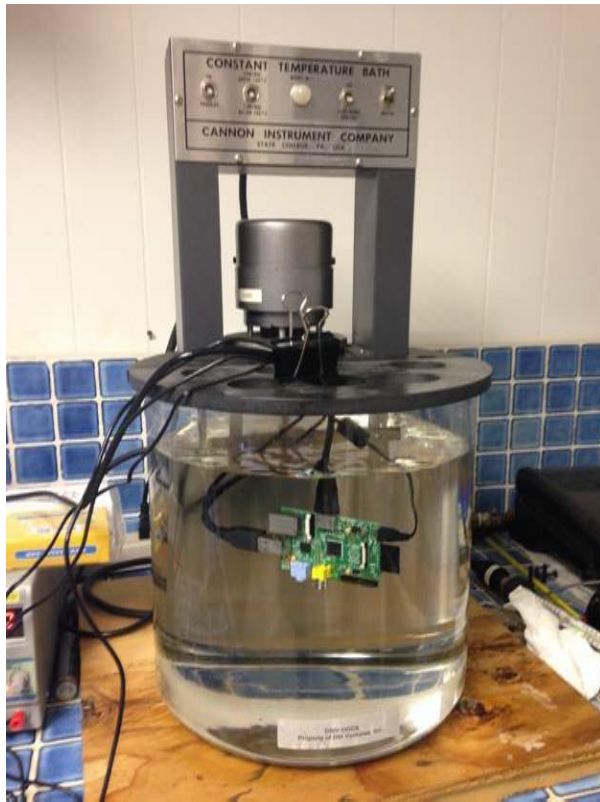
Figure 7: Raspberry Pi immersed in Opticool Fluid and powered up for temperature measurements.
