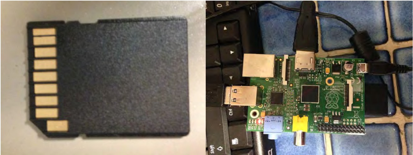
Figure 2: SD Card and Raspberry Pi condition after 6-month operation in Opticool Fluid
