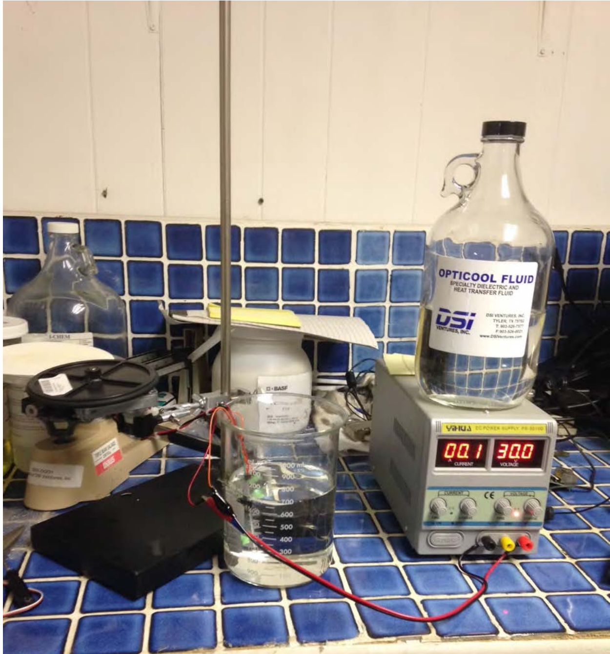
Fig 5. Motor Driver 2 immersed in dielectric cooling fluid at startup
