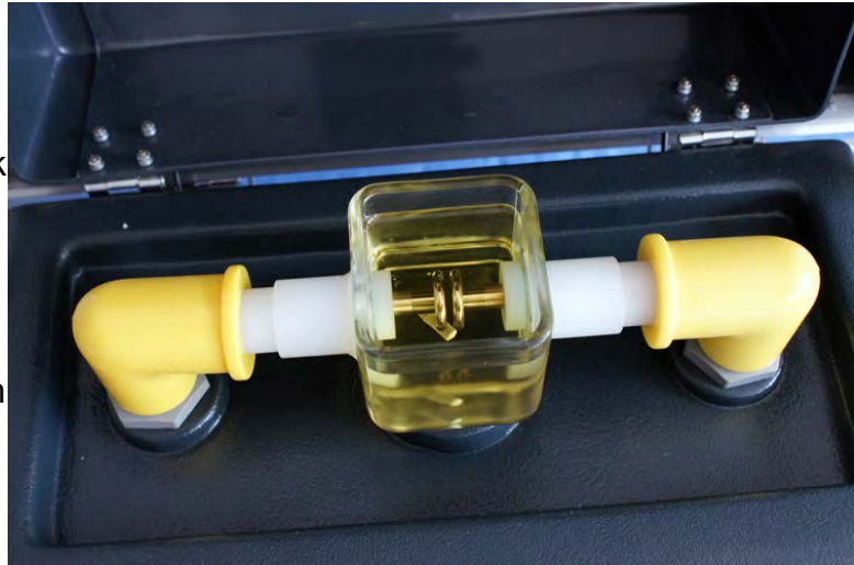
Illustration 1: Dielectric Strength Testing of Coolant
