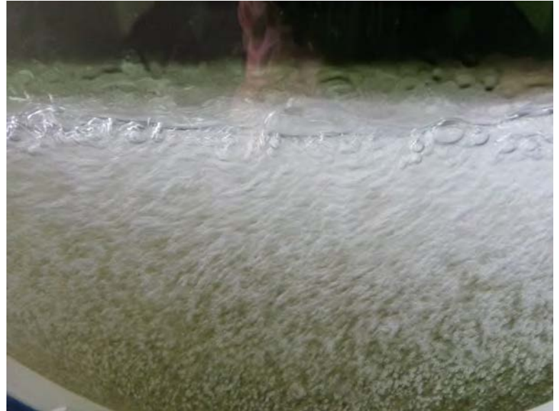
Dielectric in Vacuum Degassifier
